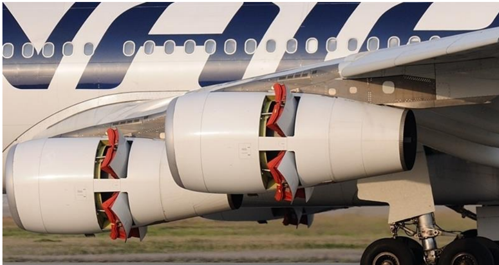
Figure 10 - Pivoting-door thrust reversal on an A340-300
